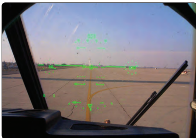
Figure 5-13. HGS using a holographic display.
