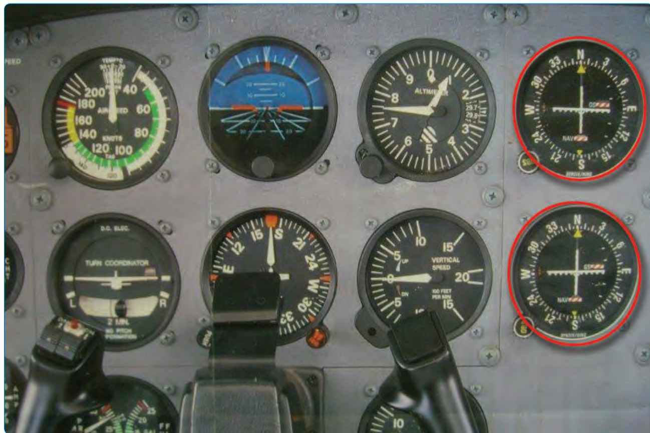
Figure 2-52. Instrument panel with dual VORs.
