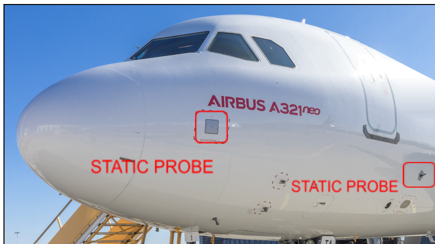
Illustration A3-1: Example of pressure probes location on aircraft
