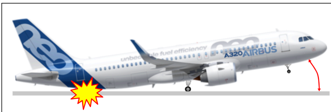
Illustration A-5: V_{MU} Demonstration (Geometrically-limited Aircraft)
