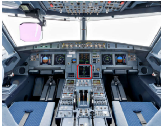
Illustration A2-2: Example of TAT and SAT location on the system display page of the ECAM
