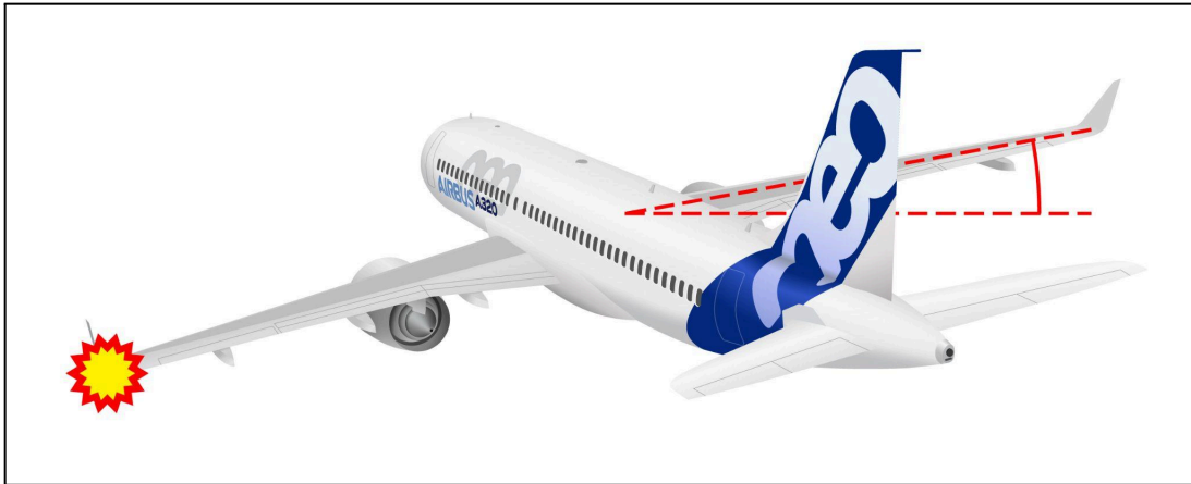
Illustration A-6: V_{MU} Risk of Wing in Contact with the Ground
