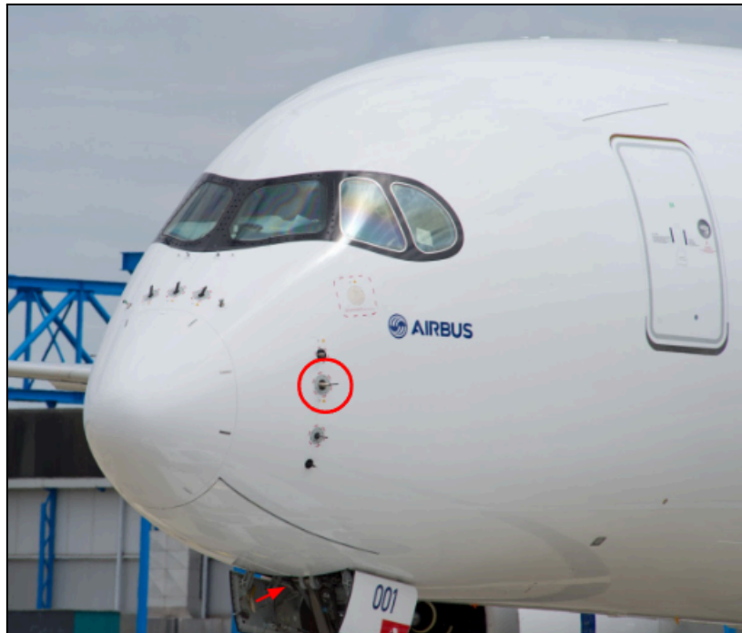
Illustration A2-1 Example of TAT and OAT probes location on aircraft
