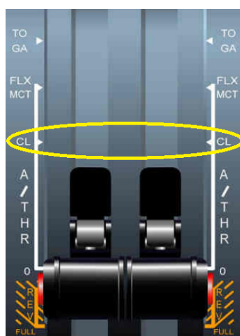
Illustration D-28: CL Gate is the Thrust Throttles Position During Descent with Auto-Thrust
