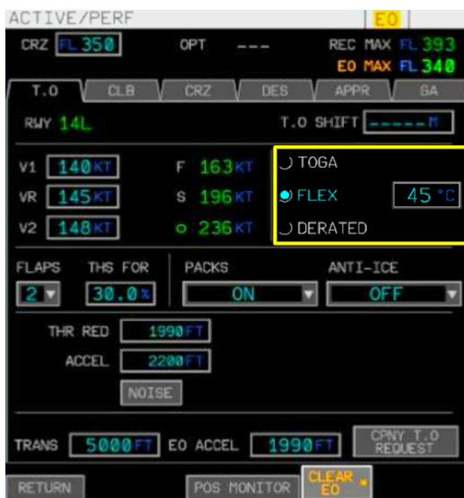
Illustration C-57: FMS Cockpit Interface Takeoff Performance
