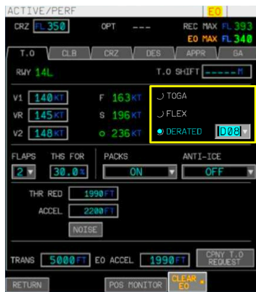
Illustration C-59: FMS Cockpit Interface Takeoff Performance
